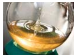
A carbon dioxide-based polymer (pictured above in resin form) has the consistency and viscosity of honey.
